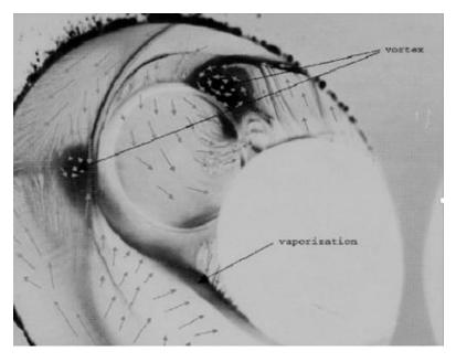
Image of vortices within a combustion chamber
