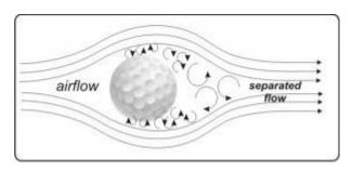
Illustration of the micro turbulence boundary layer created by dimples on a golf ball
