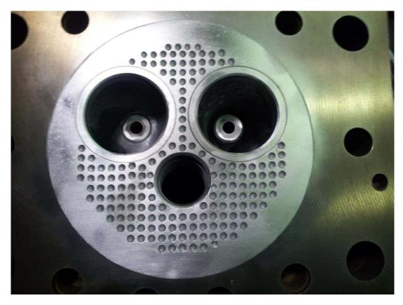
Natural gas cylinder head with dimples and ceramic thermal barrier
